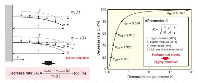
Fig. 1 Calculation model and the effect of turgor pressure on the deflection
